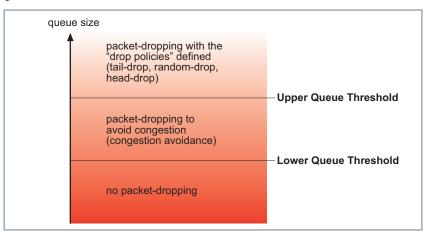
Figure 1-1: Influence of thresholds on packet-dropping
