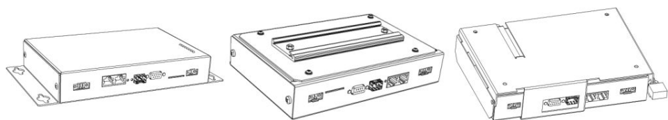
Abb. 12: Wall mounting of the bintec Wl1040n (standard design, DIN rail or theft protection optional)
