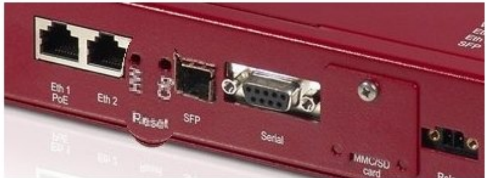
Abb. 17: Underside of the bintec Wlx040n with the HW and Cfg reset buttons
