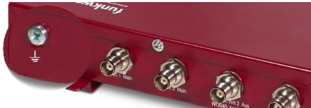
Abb. 16: Connection to earth bintec WIx040n
